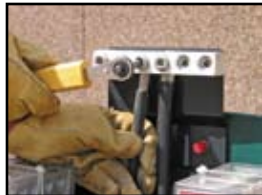
5/16" Ball-tip Hex (Allen) has a 2" working length for transformer secondary bars
