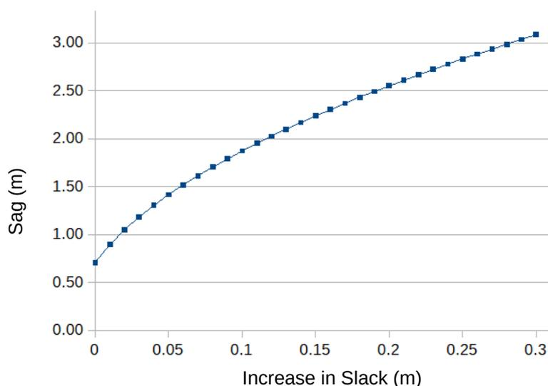
The chart shows that increasing the conductor length by 30cm increases the sag by over 2m.
