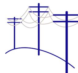
There is a relationship between the span length (horizontal distance between poles), length of conductor (also called catenary length) and sag. A small change in catenary length makes a big difference to the sag.
