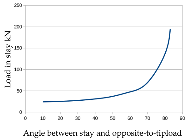
Figure 12: Tension in stay wires
