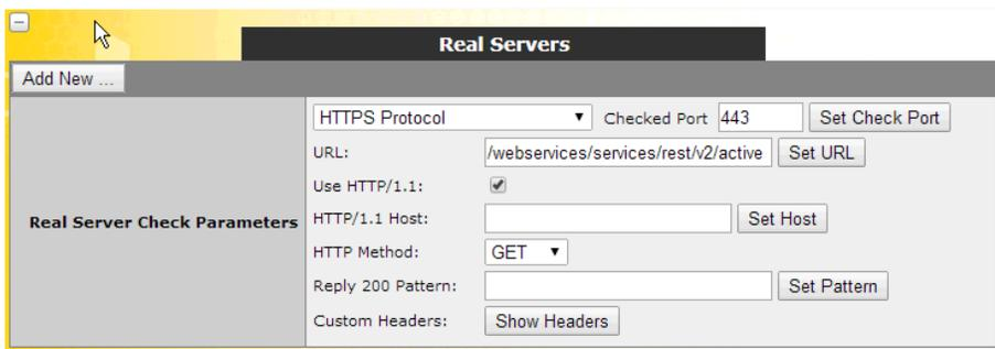
Other load balancers such as F5 require a slightly more granular configuration. In the Embotics test lab, the F5 required the send string:
