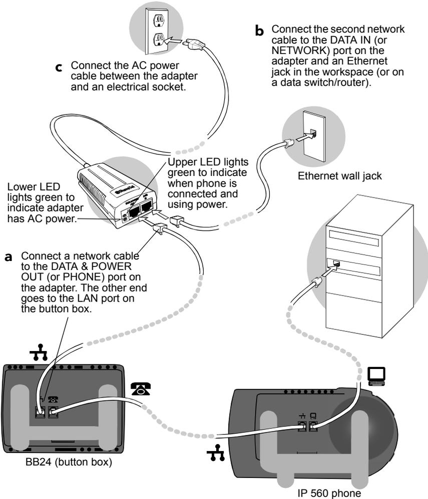
**Note:** The button box can forward power to an IP phone but an IP phone cannot forward power to a button box. Thus, if two devices will be daisy-chained, the button box must be the first device in the chain.
