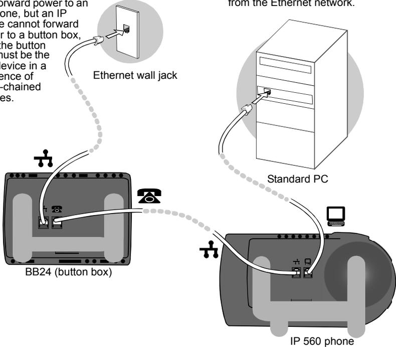
**Note:** The BB24 can only forward power to one additional unpowered device, so you cannot daisy-chain three button boxes in a row with a single powered LAN cable. If you would like to connect two or more button boxes and an IP phone, a second Ethernet wall jack is needed to provide adequate power.
