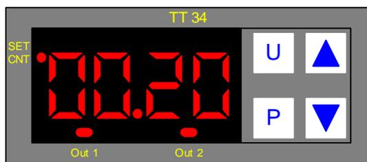
The display is used to set the required cycle time between a minimum of 00:01 and a maximum of 99:59. To adjust proceed as follows:
