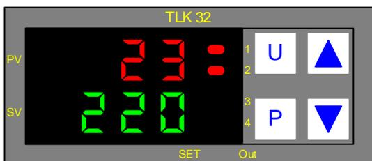
The green SV (Set Value) section of the display is used to set the required plate temperature in degrees C between a minimum of 20 and a maximum of 220. To adjust proceed as follows,
