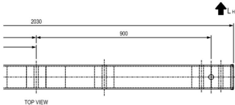
This load converts to a bending moment by multiplying it by the application distance from the pivot point. For a crossarm this is the kingbolt. The diagram shows the application point as 0.95m from the kingbolt.
