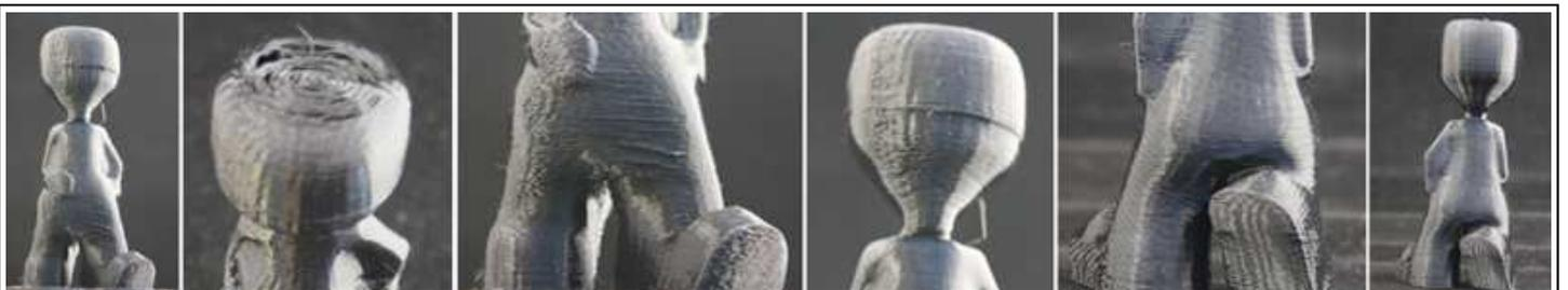
1.3 Print quality impaired without filament fan. Notice the slight droop on the foot, chin, thigh and stomach, and the hole in the head!
