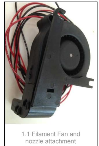
1.1 Filament Fan and nozzle attachment
