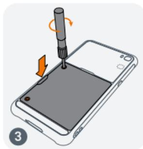
Make sure the device is turned off before replacing the battery pack. ❶ Loosen the two fasteners with the supplied Torx T10 screwdriver (the fasteners are captive screws and not suppose to be fully removed). ❷ Remove the battery pack. ❸ Replace the battery pack and tighten the fasteners.
