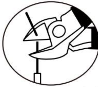
Diagram 2; trim any wire in excess of 5mm / 0.27".
