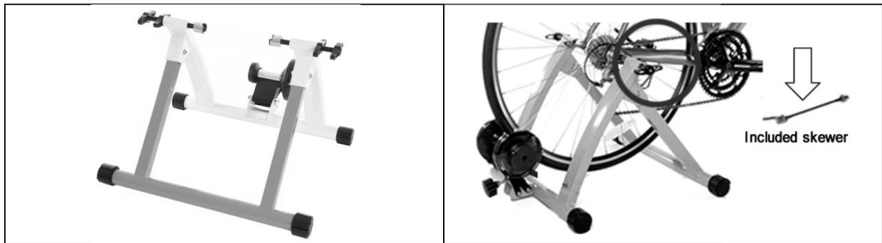
1. Remove all packaging, unfold the frame, and place on a level floor. Twist plastic feet (numbered 1-5) on ends of base to desired level; adjust as necessary for uneven floor.
