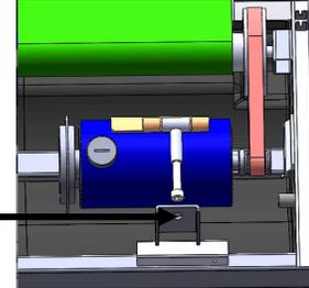
Fig. 6, adjusting bolt
