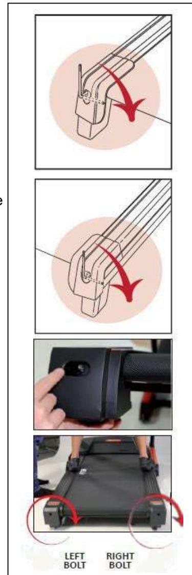
4. Tighten the treadmill's belt (if the belt slips on the treadmill when walking). Start treadmill and increase the speed to 3/mph. Using the 5mm Wrench, turn both bolts 1/4 clockwise (Fig. 4, 5). To see if the belt is properly tight to walk, you should be able to pull up each side of the belt 5 or 7 cm off the platform. Be careful and keep the belt aligned. Repeat this procedure until the belt is properly tightened.
