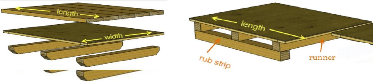
**Medium Duty Base:** Runner components will run left-to-right (length). Uses Rub Strips that are segmented and run parallel to the Runners (skids). Rub strips are segmented to allow for fork lifting from the front and usually allow for sling lifting. If the crate's length is small enough, there may only be one rub strip.
