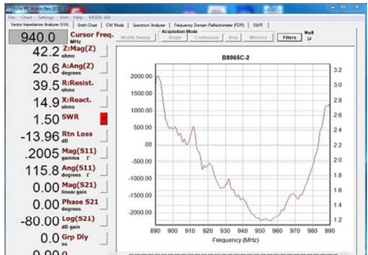
Echo Test antenna #2 with Cable Null ON to eliminate the test lead
