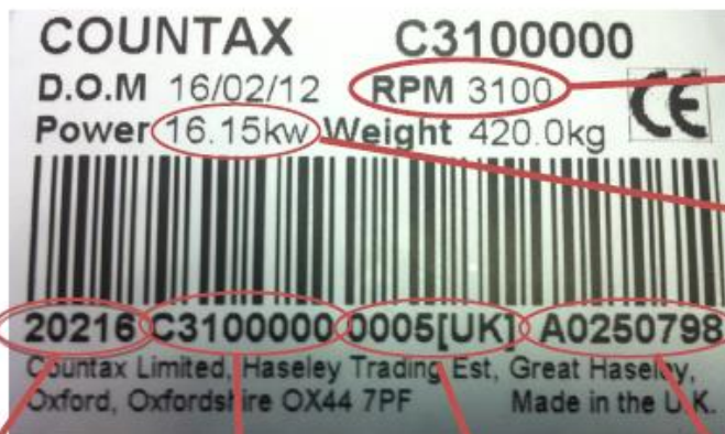
On the under side of the chassis, behind the axle
