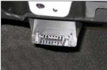
Figure 12: Re-mounted OBD-II Port Connector
