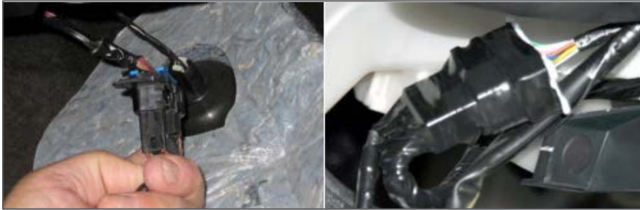
Figure 11: Plugged OBD-II Connectors and Taped Connectors
