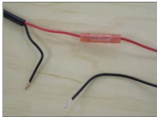
Figure 9: Connect Power and Ground using supplied connectors
