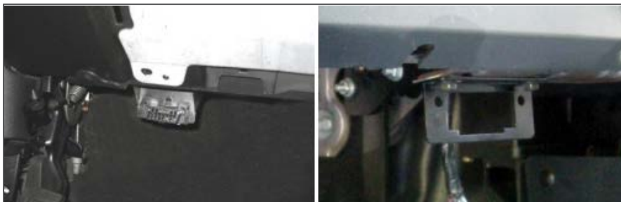
Figure 10: Vehicle OBD-II Port Connector and OBD-II Flange Mounted
