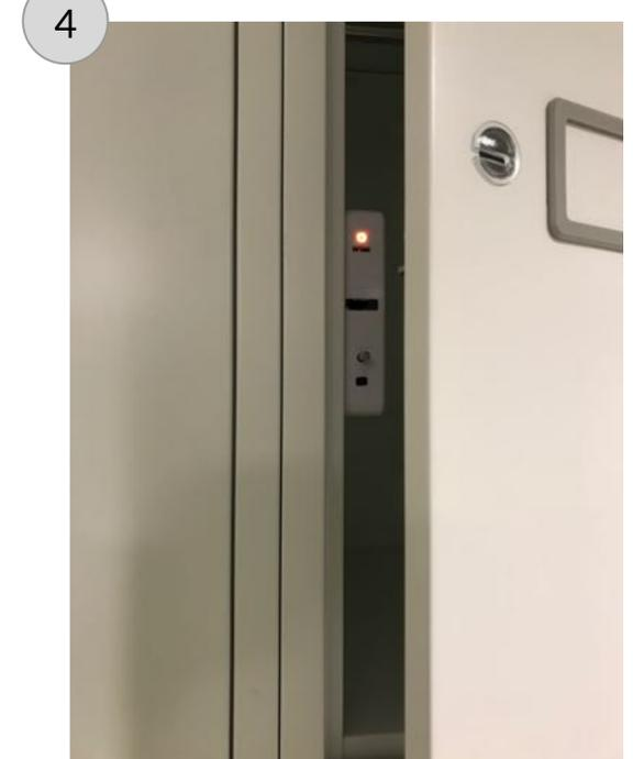
Swipe a card that is known to work or otherwise attempt to open a locker via the Smartlock App or kiosk PIN code. Watch for the door to open.
