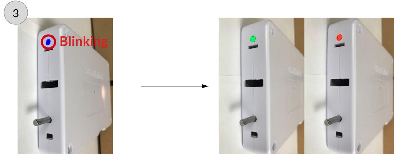
When the PoE injectors are reset, each locker will transition from Blue blinking to either Green or Red (depending on whether the locker is reserved or free).
