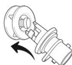
Figure 2 Insert locking pump connector
