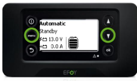
🔌 Press the [menu] and [▼] button on the remote control panel at least 3 seconds
