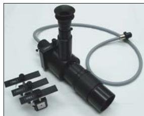
This device images the measurement plane onto an aperture; light incident on the aperture is output for measurement, the remainder of the view is reflected up to an eye-piece. In this manner, the user views a scene with a black spot corresponding to the area being measured.
