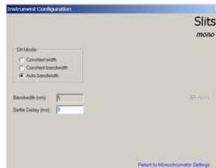
*It should be noted that having calibrated a system in auto mode at a given step size, to change the step size would invalidate the calibration.*
