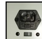
At Bentham, the appropriate fuse (plus a supplement) is fitted. Should the voltage setting be wrong, please ensure that the correct fuse is installed.
