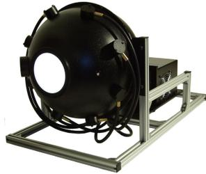
Light is coupled from a 250W quartz halogen lamp with an ellipsoidal reflector, and is transported to a 300mm diameter integrating sphere, coated with barium sulphate, via an 8-branch fibre for homogenous illumination. Between the lamp and the fibres is situated micrometer adjustable bi-lateral slits to vary the light level, variable over 50 $\mu$ m to 10mm.
