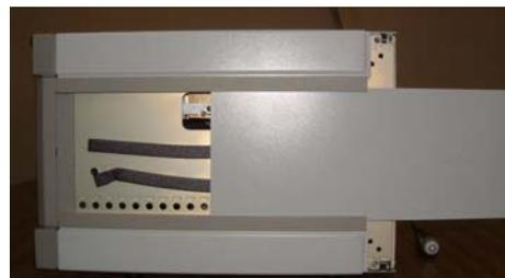
Figure 5:- Removing central trim panel to expose alignment screws
