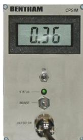
The CPS1M is connected to the Peltier cooled device via Amphenol socket.
