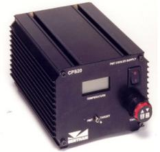
On the front panel there is a toggle switch and a rotary switch. The toggle permits to go between displaying the actual and target temperature; the rotary switch permits changing the target temperature. This latter switch should be pulled out before rotation, and pushed-in to lock the position.
