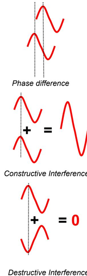
Figure 6:-Wave interference
