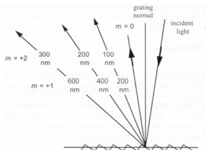
Figure 10:- Existence of diffraction orders
