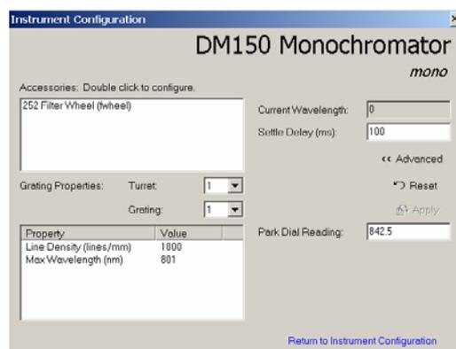
The park dial reading obtained from the wavelength calibration certificate should be input.
