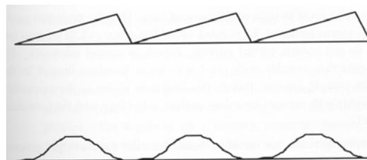
Figure 11:- Groove shape obtained using ruling (upper) and holographic techniques
