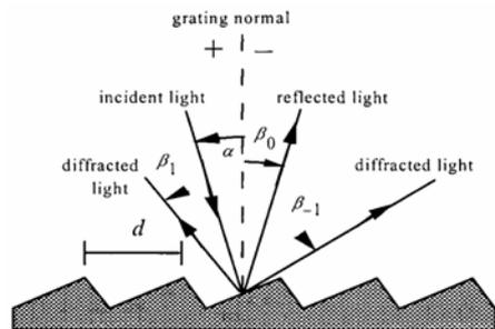
Figure 8:- Plane reflection grating diffraction
