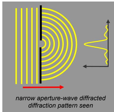
Figure 7:-Single slit diffraction
