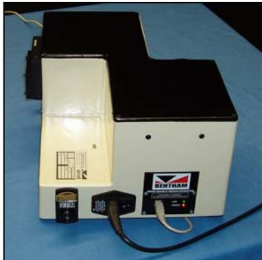
Figure 1:- DMc150F-U monochromator
