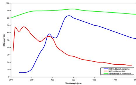
Figure 12:- Example grating efficiency curves
