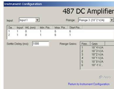
There are two setups, for which the properties may be defined. In multiple detector setups, the start wavelength of the second setup should be defined.
