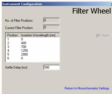
The insertion wavelength relevant to the filter in a given position should be input. The order need not be ascending.
