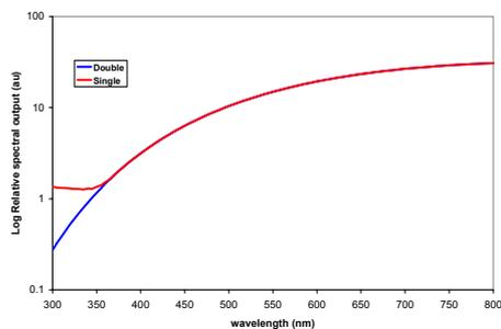
Figure 14:- Measurement of QH lamp with single and double monochromators
