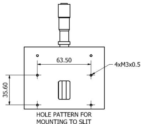
Figure 3: TMc150 slit hole pattern
