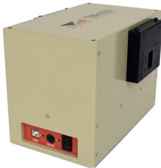
Figure 1:- TMc150 monochromator
