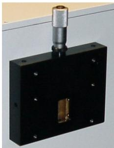
Figure 5:-Micrometer variable slit
