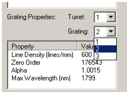
The zero and alpha parameters for each grating are obtained from the calibration certificate.
