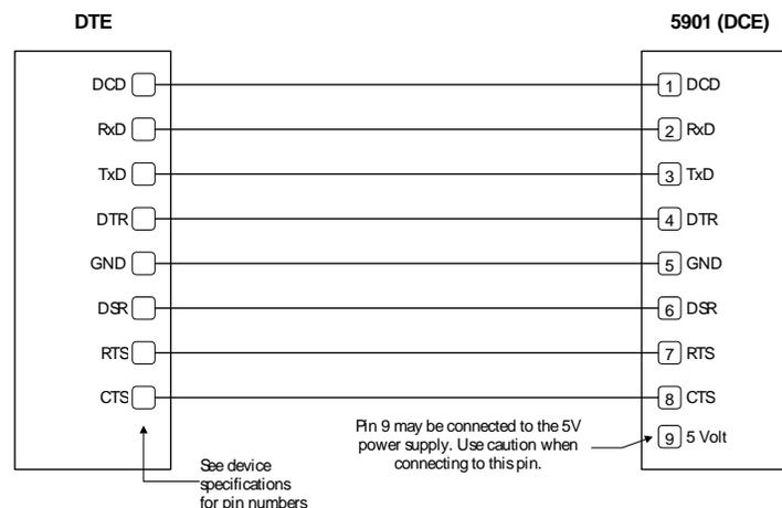
**Figure 3: RS-232 Wiring - 5901 (DCE) to DTE**
