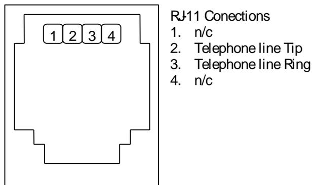
**Figure 4: 5901 Modem RJ-11 Connection, P6**
