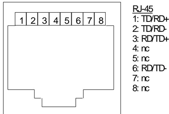
Figure 2: 5905 Ethernet RJ-45 Connection
