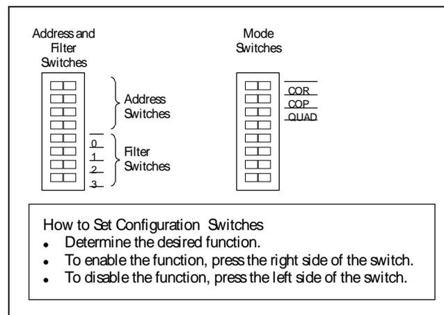
**Figure 4: Configuration Switches**
