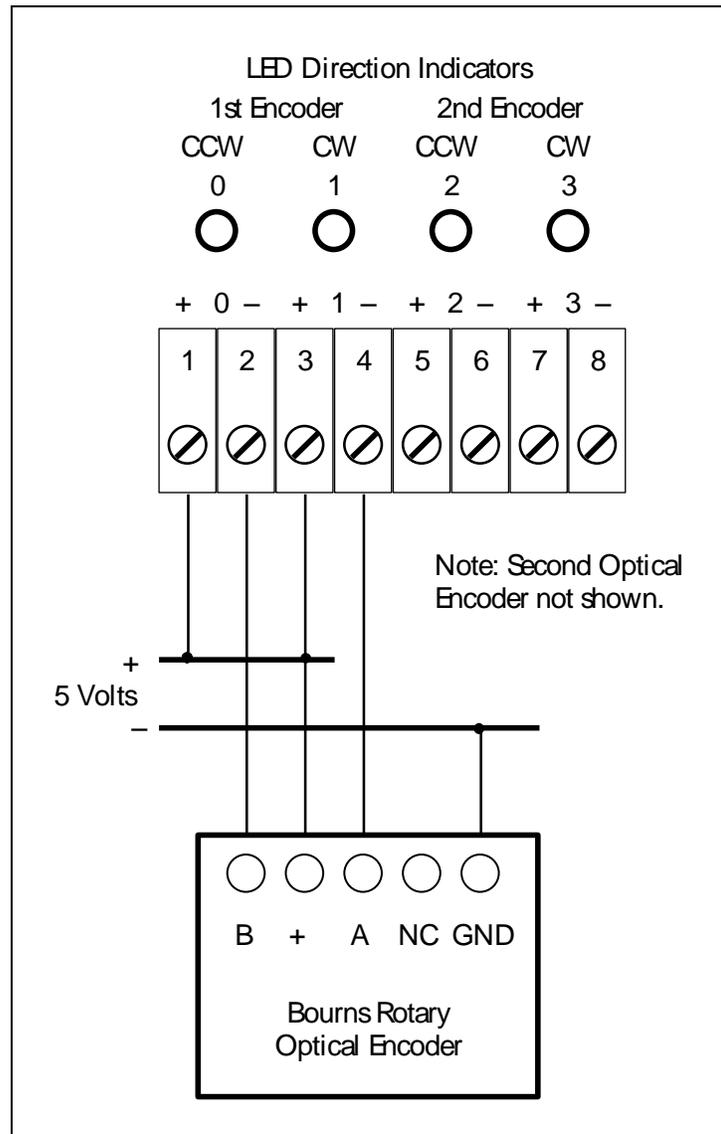
**Figure 2: Optical Encoder Wiring Example**
