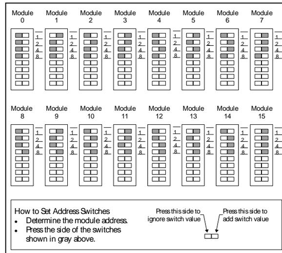
**Figure 3: Model 5410 Module Address Switches**
