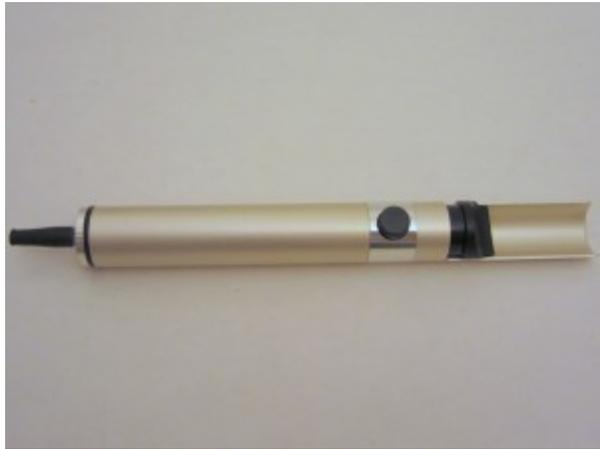
**Solder sucker (desoldering pump).** Similar to above but does not come with a heating unit. This is more common but not as easy to use nor as effective.
