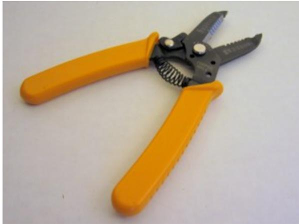
**Wire stripper and cutter.** Generally useful for cutting and easy stripping wires of different sizes.
