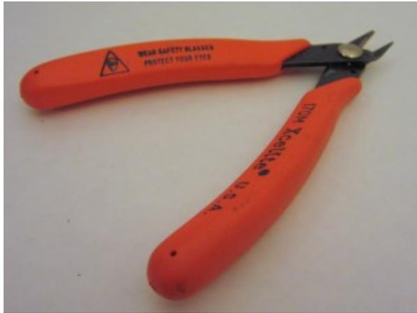
**Shear cutter or diagonal cutter.** Essential for cutting leads close to the PCB. A must-have tool for soldering through-hole components. Instead of buying it alone, I recommend getting a 'mini pliers tool set', which includes the cutter and other useful pliers.
