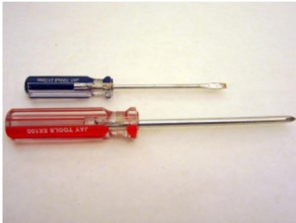
**Screwdrivers.** You need a couple of basic screwdrivers to fix the board to the enclosure, and to fix sprinkler valve wires to the terminal blocks.
