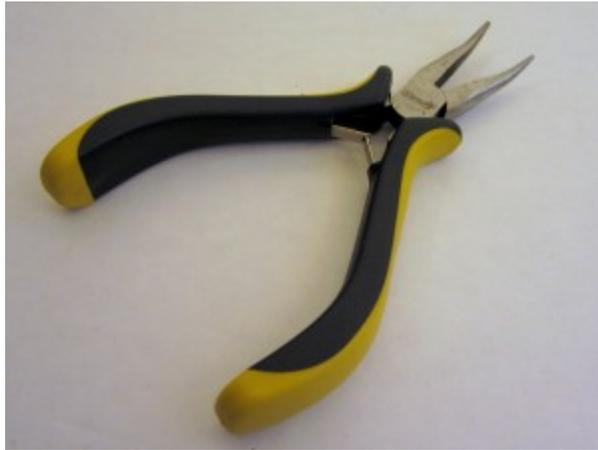
**Pliers.** Needle nose pliers or flat nose pliers are useful for bending component lead. As mentioned above, I recommend getting a mini pliers combo set such as [this one](#).
