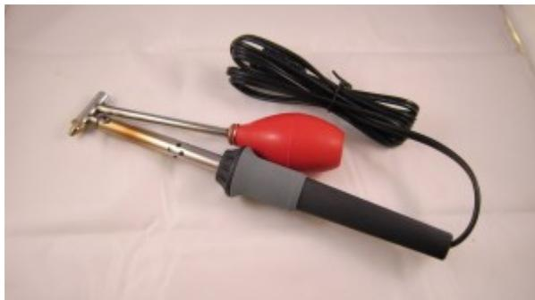
**Desoldering Iron.** For taking components off PCB and fixing soldering mistakes. This one is from [RadioShack](#). It has 45W power and a rubber bulb. Cheap and handy. Best desoldering tool I've used.
