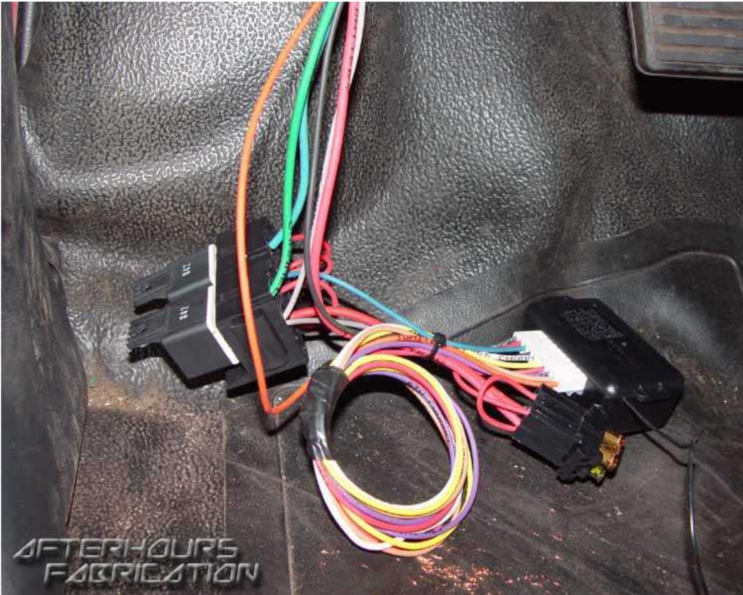
Heres a shot of where I typically hook up the source for the brain. This is a 2003 S-10 so the pink wire under the column is tapped for voltage. Remember to check the wire with a multi meter tho.
