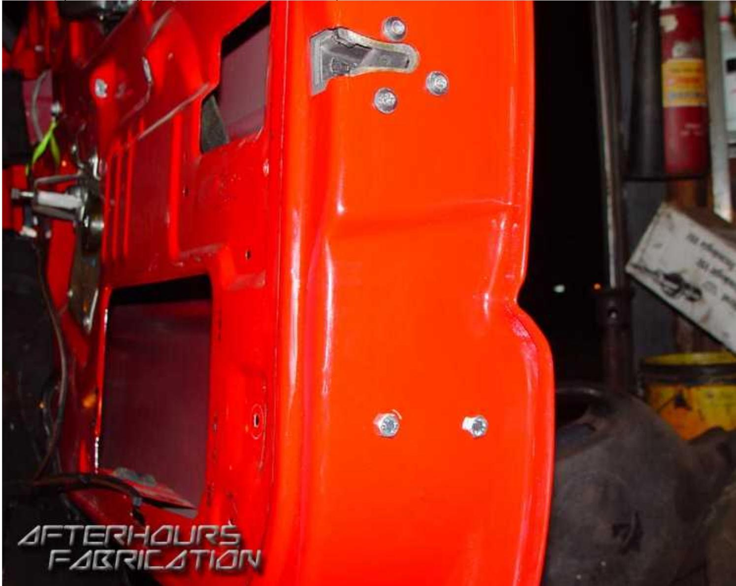
I then measure the distance from the top of the [solenoid](#) to the latch mechanism, then pull the latch and actuator out, set them down the right distance apart, and run the steel cable thru both and crimp the supplied cable stay in the middle. Its much easier this way then trying to work inside the [door skin](#).
