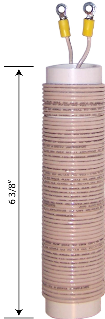
39 turns around 1 1/4" PVC pipe
