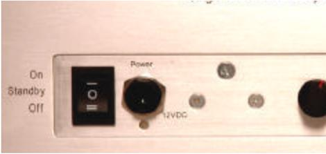
3. Connect AC power supply cord to “Power/ 12VDC” port on console, then plug into AC outlet.
