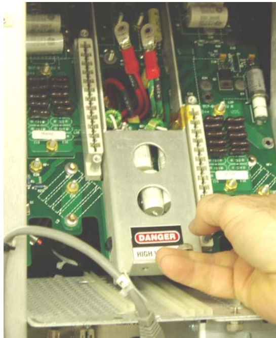
Figure 15 – Tilt Motherboard into Vertical Position
