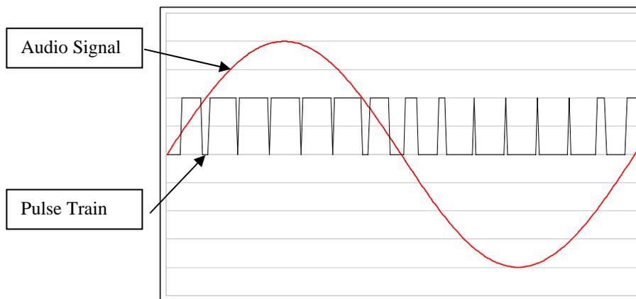
Figure 2: PWM Generator Pulse Train
