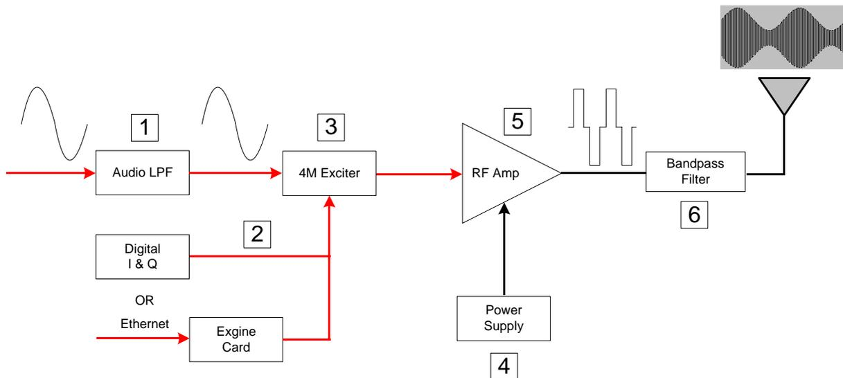
**Figure 4: 4MX Transmitter Diagram**
