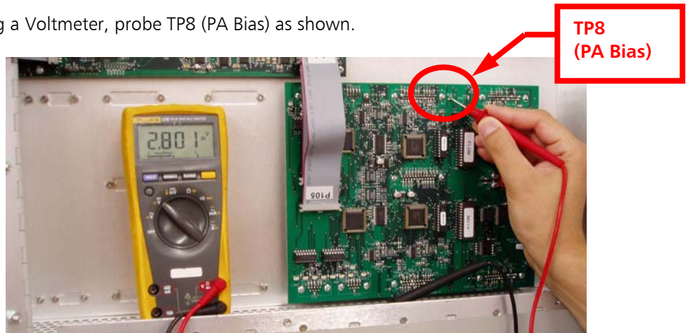
Figure 5 – TP8 (PA Bias Voltage)
