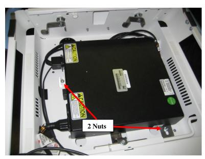
1) Remove 2 nuts shown, securing inverter.
