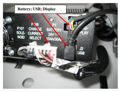
3) Unplug Battery, USB and Display cables shown.
