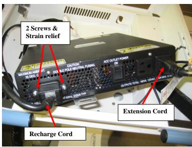
2) Lift inverter, remove 2 screws shown and remove strain relief with recharge cord. Unplug extension cord. Note: Screws, strain relief and extension cord will be reused. Some newer revision carts do not have strain relief.
