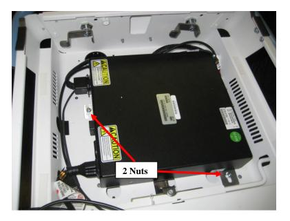
7) Position new inverter in place and secure with 2 nuts as shown.
