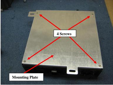
4) Remove mounting plate from old inverter and install onto new one with 4 screws shown. Be sure orientation is correct.
