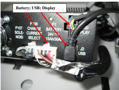
5) Plug in recharge cord with strain relief, secure with screws removed in step 2. Plug in extension cord.
