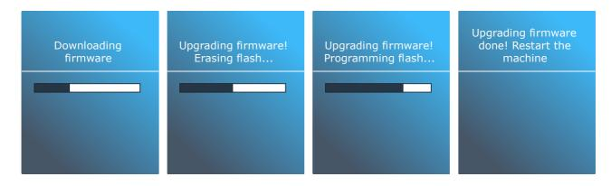
Reboot the machine to finalize the firmware upgrade when the display instructs to do so.
