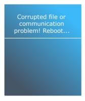
In case an incorrect firmware file was sent to the cutter, then an error message is displayed:
