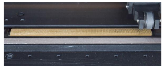
Cleaned drive drum
