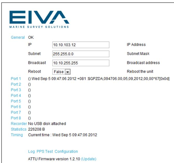
Figure 3: Setup using the unit's web interface. Showing the general tab expanded and the port menus listed below.
