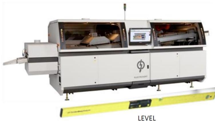
6. Adjust the front load and unload leveling legs until the level indicates proper positioning.
