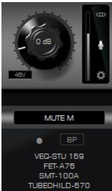
This is a single mic/combo input with a gain adjustment knob, controls, and peak metering. There are four such inputs for the Discrete 4 Synergy Core and eight for the Discrete 8 Synergy Core. Below the preamp controls, you see an Input Selector (where it says 'MUTE M') and an AFX area.
