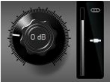
Make sure your input looks like this and adjust gain as required. The 'Connector' symbol means an input is configured to accept line-level signal.
