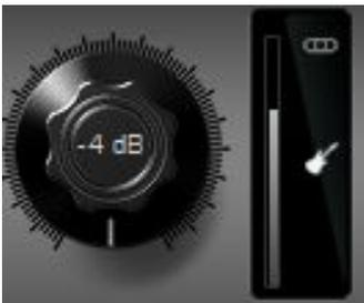
Make sure your input looks like this and adjust gain as required. Hi-Z inputs are available on Discrete 4 Synergy Core mic/combo inputs A1 and A2, and on Discrete 8 Synergy Core preamp/combo inputs A1 to A4.
