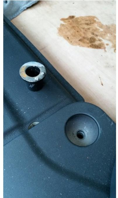
File or drill the rear right-hand seat mounting hole to accept the larger bolt that is supplied in this position.
