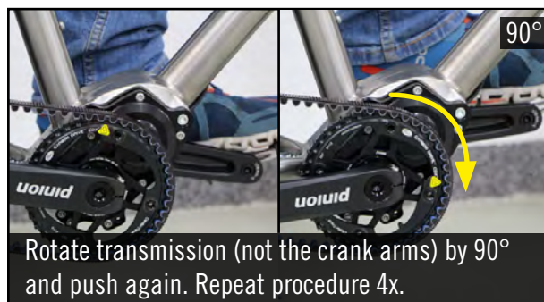
Shift into first gear and apply rear brake. Place foot on horizontally positioned pedal and push.
