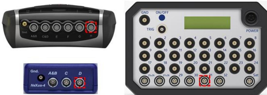
Sensors can be disconnected by pulling the silver ribbed part of the connector backward.
