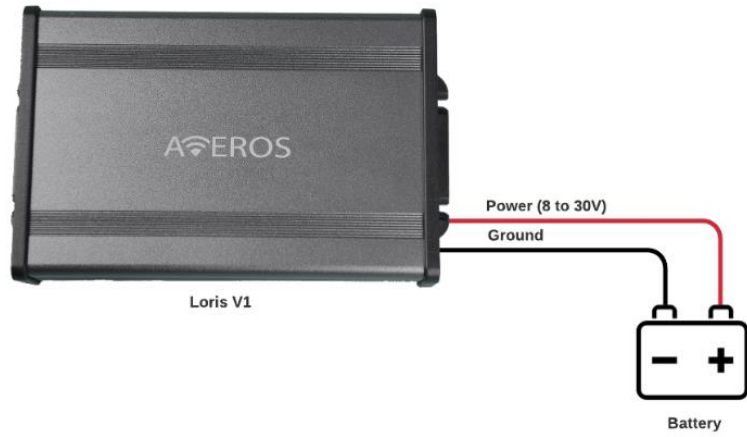
Figure 11 Loris V1 Wiring
