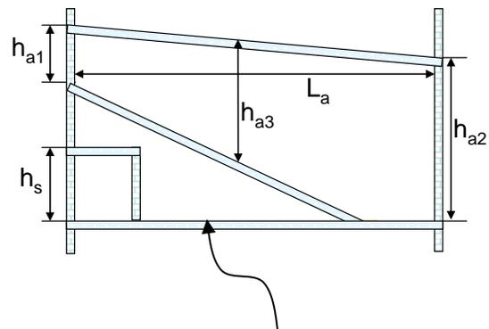
Don't forget this void is another zone if it has a different activity! Its zone height = area weighted average vertical wall height. If it has the same activity or is inaccessible, then merge with auditorium and enter zone area as though the floor is flat ( $L_a \times d$ ). However, the sloping floor area must be input so that thermal mass is calculated.)
